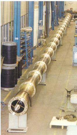
Typical applications for centrifugal castings include cylinders for compressors, engine liners, valve and pump components, propulsion and launch systems and rings and seals for gas turbines. Spunalloys also produce column pipe assemblies which can be many metres in length (pictured).
