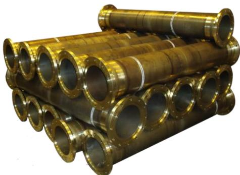
**Figure 4:** Centrifugally cast, weld-assembled and finish machined column pipes ready for despatch to the end client. Fully traceable to individual heat number cast, and certified to customer requirements.
