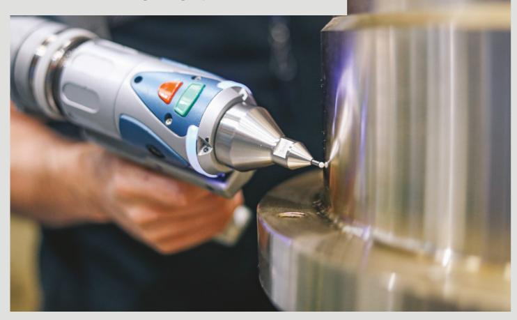
A technical team of fully trained and qualified metallurgists is responsible for material analysis, ensuring materials meet the chemical requirements of every order. We use certified high-quality ingots from reputable material suppliers, and on melting, a melt button is taken from every furnace charge to be checked in one of our on-site electron emission spectrometers.
